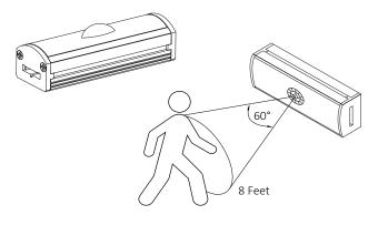
When motion is detected, sensor switch will illuminate attached LED load. Continuous motion will keep lights activated. Lights will shut off 10 seconds after motion is not detected.
